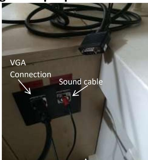
Connect your laptop to the provided VGA and sound cable. One end will plug to the connectors provided and the other end to your laptop.
